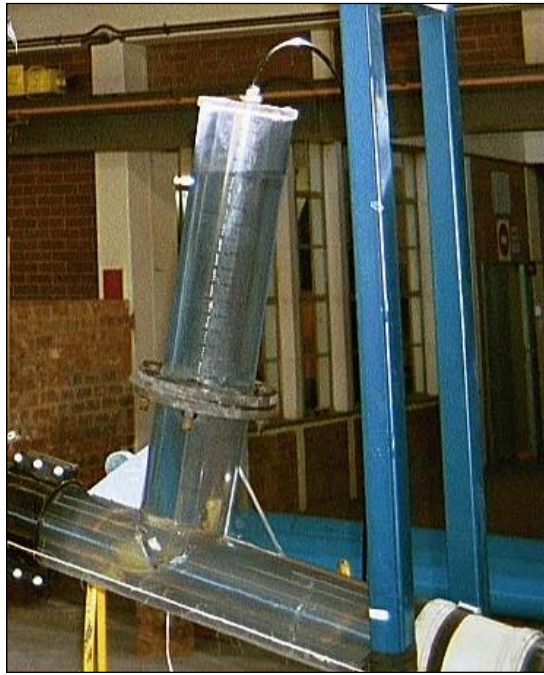
Figure 5: Vertical off take pipe used in Test 2
